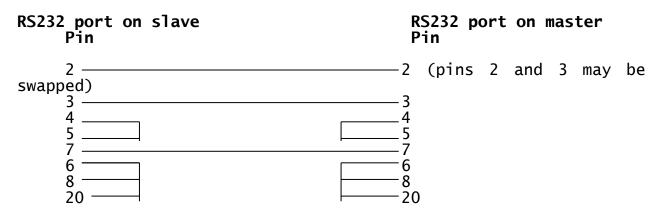
Pins 4 and 5 are connected together at each end of the cable as are pins 6, 8 and 20.
